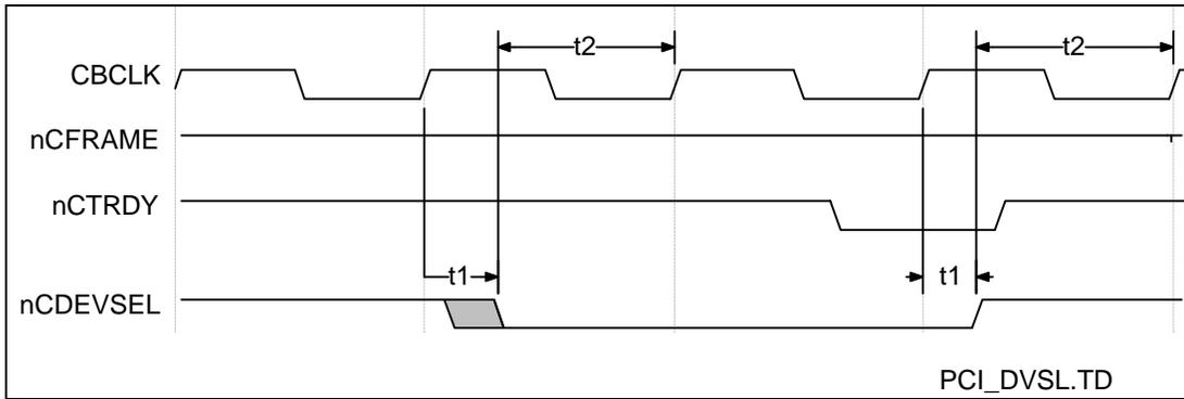
**FIGURE 7 - CardBus/nCDEVSEL TIMING**
