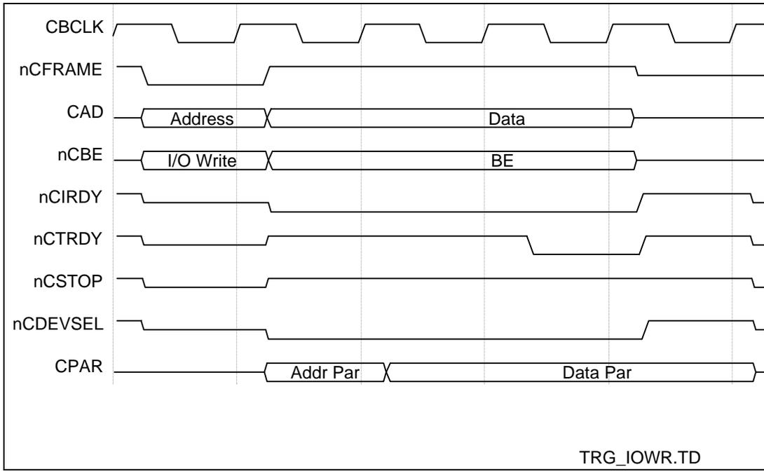
**FIGURE 14 - CardBus - TYPICAL I/O WRITE/EPIC/C IS TARGET**
