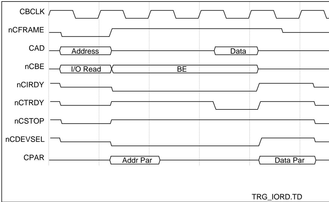
**FIGURE 13 - CardBus - TYPICAL I/O READ/EPIC/C IS TARGET**
