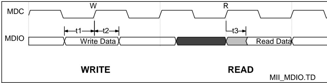
**FIGURE 20 - MII - SERIAL MANAGEMENT WRITE/READ**
