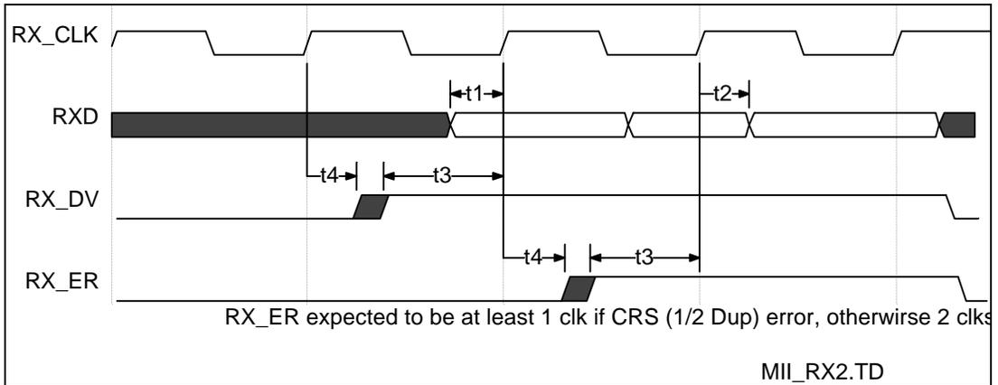
**FIGURE 19 - MII - RECEIVE ERROR (RX\_ER) TIMING FOR 100Mb/s**
