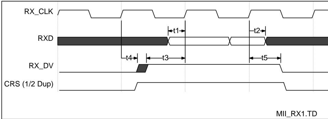
**FIGURE 18 - MII - RECEIVE TIMING FOR 100Mb/s**
